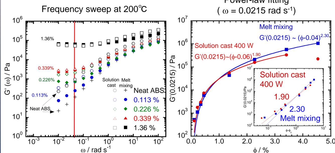
**Electrical Conductivity:** Melt mixing using an internal batch mixer is at least as good as solution casting!
