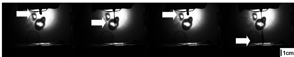
Fig.1 Returning behavior after falling down certain distance under applied Electric Field. Image is captured at 0.0sec, 2.0sec, 2.1sec, 8.3sec ( from left side ) after starting capture images ( Voltage is applied at 1.2sec).
