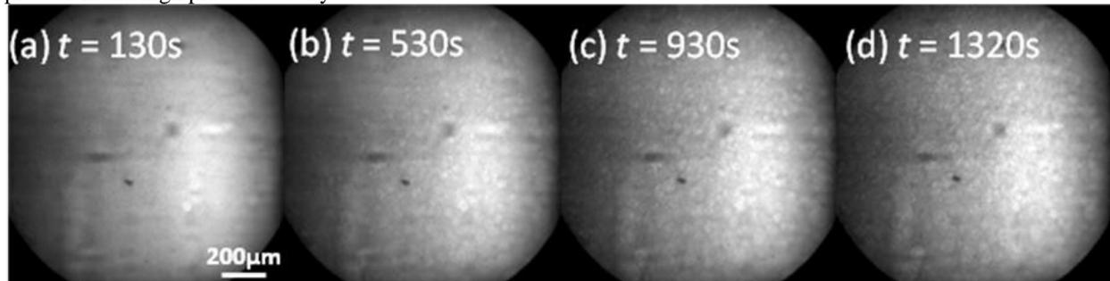
**FIGURE 2** A series of X-ray transmission image of one-shot chemical foaming process at 433 K (a-d).
