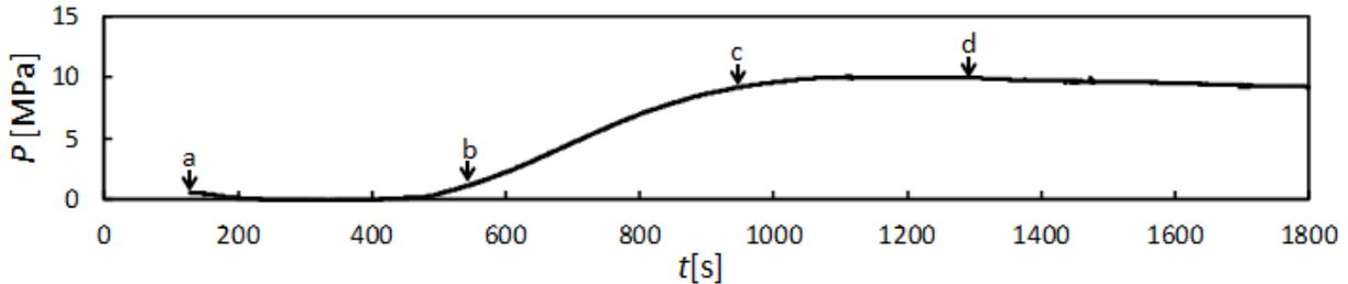
**FIGURE 1** Cavity pressure profile of LLDPE compound at 433K. Arrows denote the timing corresponding to images of Fig. 2.
