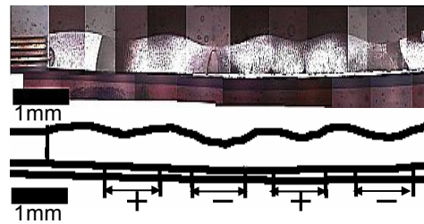
Fig.3 Optical micrograph of cross section V=4\text{ kV} , Initial thickness: 330\mu\text{m} Scale bar: 1 mm, Image is magnified two times in vertical direction.
